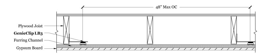
Note: Minimum of 1/8" spacing between Plywood Joist and Furring Channel
