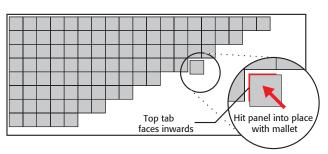
Do not directly hit the edge of the **GenieMat FF** panels with a mallet or hammer. Use a wood block flush with the edge to distribute the load and protect the edges as the panels are hit into place.
