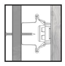
NOTE It is impossible to "short circuit" the **GenieClip RST**System when the correct screws are used. Should the installer hit a clip location, they will not be able to 'seat' the screw. They will be forced to move left or right on the track away from the **GenieClip RST**.
